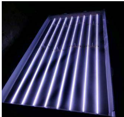
CCFL backlight unit for a TV (Old technology)
