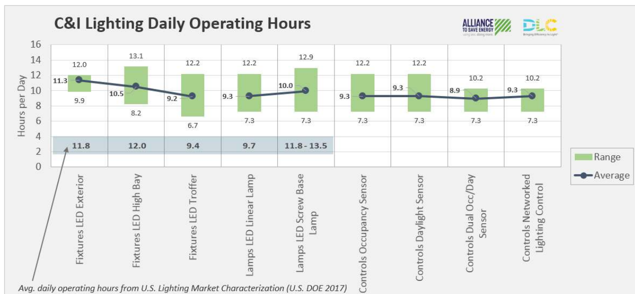
Figure 6: C&I Lighting Daily Operating Hours
