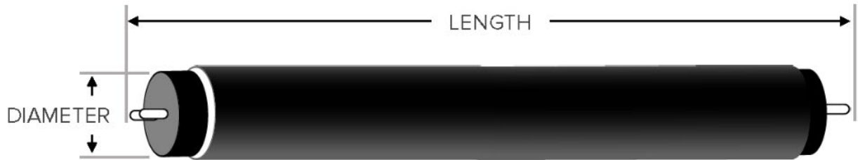
Figure 3. Dimensions of linear replacement lamps to be reported on the application form.
